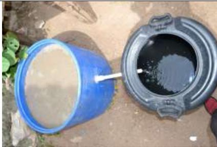
Grey water passes through the sand layers and gets into the receiving container through the pipe.
