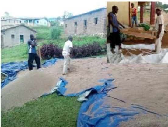
Sand sieving and sorting according to the recycling layers
